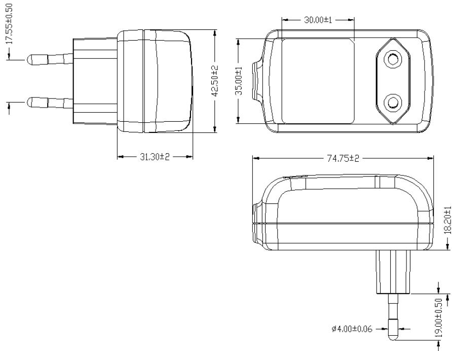
Enclosure Type: PC Temperature: 120°C 94V0
