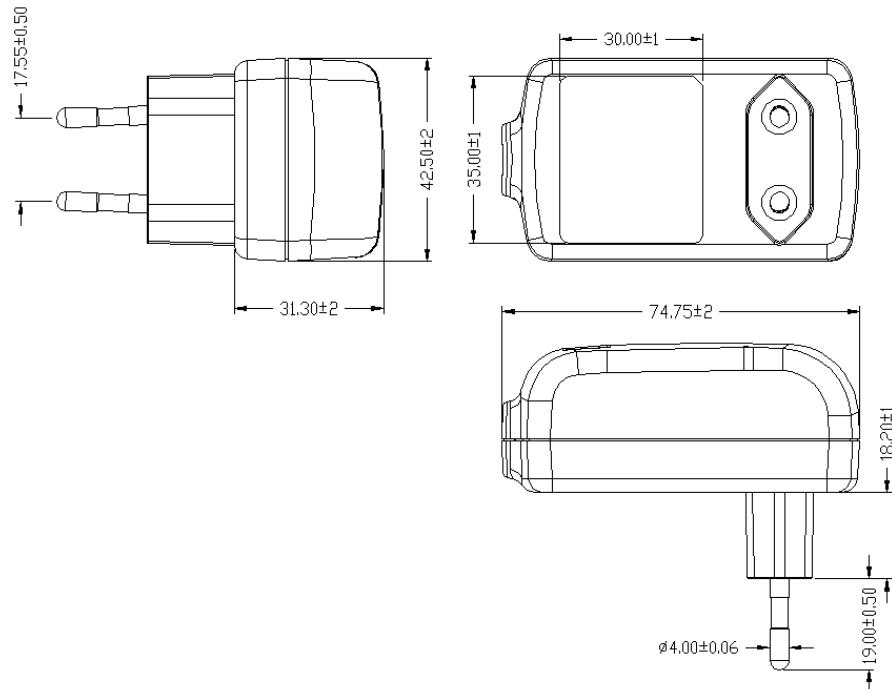
Enclosure Type : PC Temperature: 120°C 94V0
