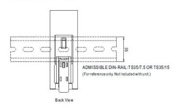
This series fits DIN-RAIL TS35/7.5 or TS35/15. For installation details, please refer to the USER MANUAL on http://www.meanwell.com/search/EDR-150/EDR\_manual.pdf
